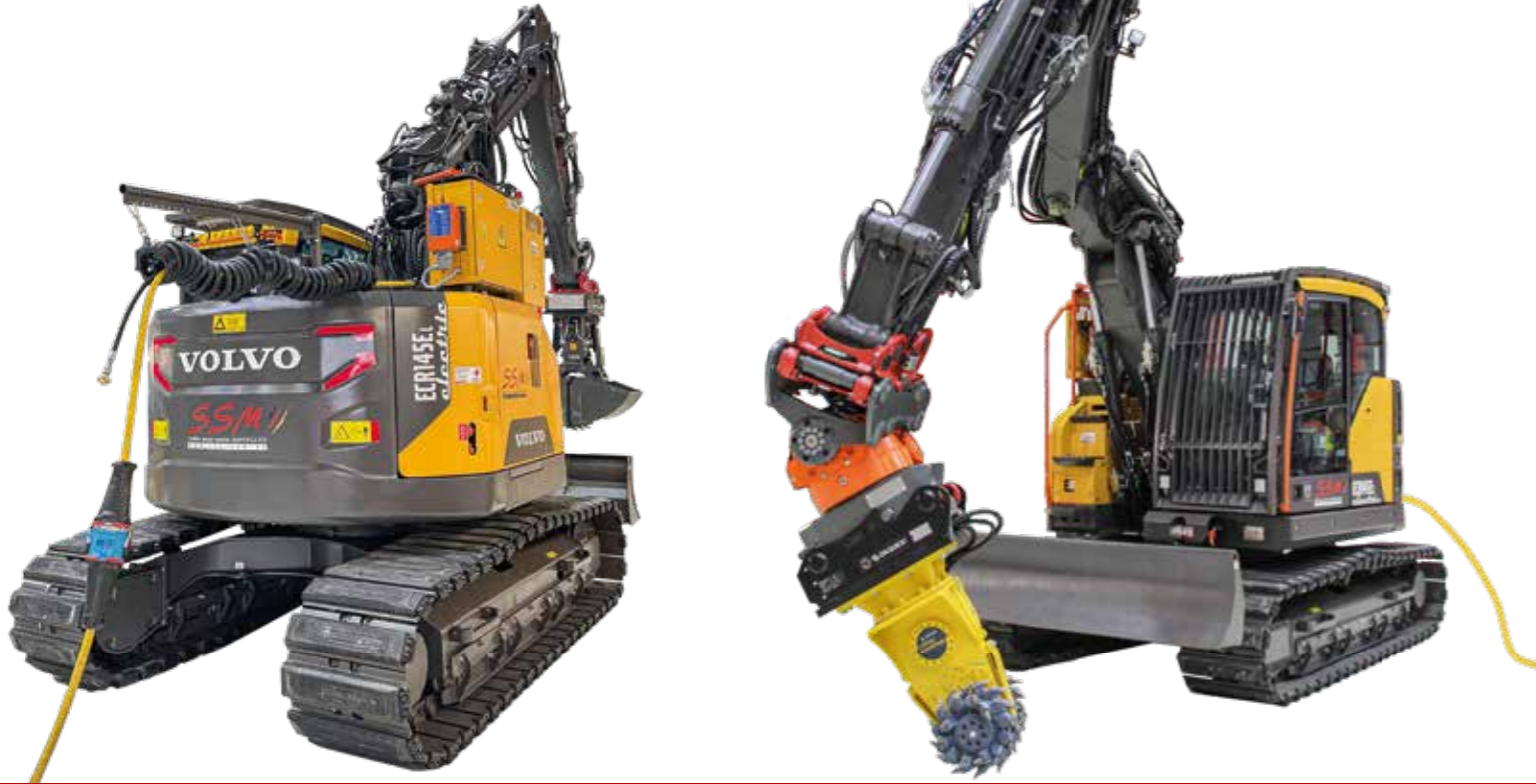
ECR145E with electric drive and radio remote control (power feed on the upper carriage)
