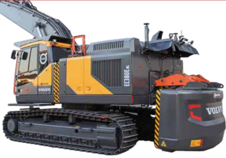
Hydraulically detachable rear counterweight
