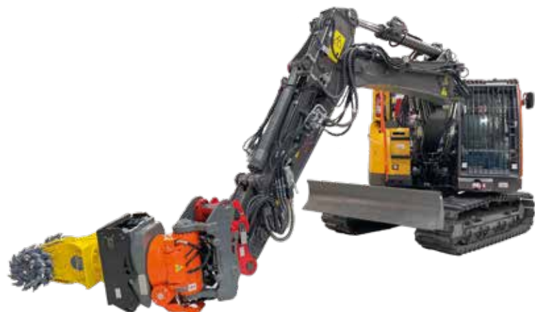
Laterally adjustable offset-boom
