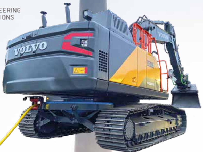
EC300E with dual drive (cable reel at the undercarriage)
