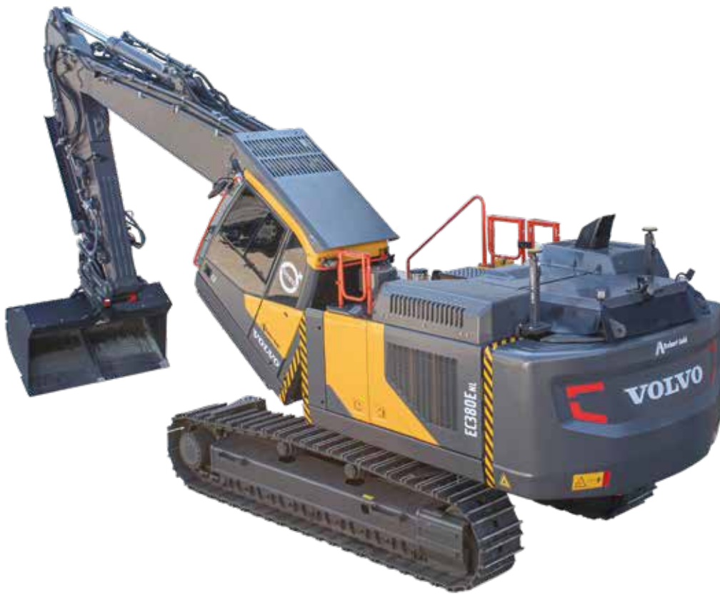
Tiltable cab and straight boom
